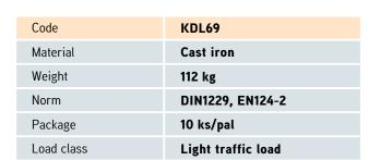
cover without hinge, horizontal PUR shock-absorbing lining on frame, horizontal and vertical PUR shock-absorbing lining on lid, without spring-loaded lid locking in frame
