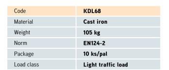
cover without hinge, horizontal PUR shock-absorbing lining on frame, horizontal and vertical PUR shock-absorbing lining on lid, without spring-loaded lid locking in frame
