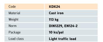
cover without hinge, horizontal PUR shock-absorbing lining on frame, EPDM shock-absorbing lining on cover, without spring-loaded lid locking in frame
