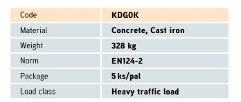
cover without hinge, horizontal PUR shock-absorbing lining, without spring-loaded lid locking in frame
